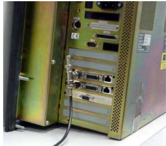
11. Attach one end of the CAT5 cross-over cable (508986) to the end of the fish tape, using electrical tape to secure the connection. Gently pull the cable back through the highflex conduit, leaving at least 5-6 feet of cable beyond the end of the conduit that will be routed through the touch screen swing arm.
